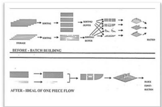
Gambar 3.2 Batch Processing vs One-piece Flow(Jeffrey Liker,2001)
